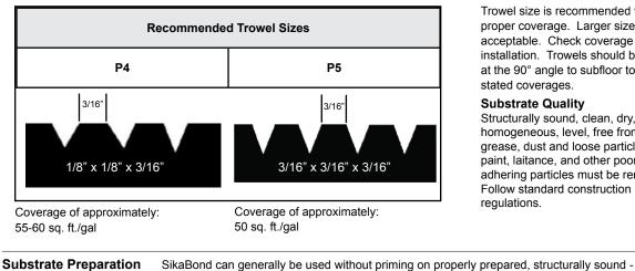
Trowel size is recommended to obtain proper coverage. Larger sizes are acceptable. Check coverage during installation. Trowels should be used at the 90° angle to subfloor to get stated coverages.
